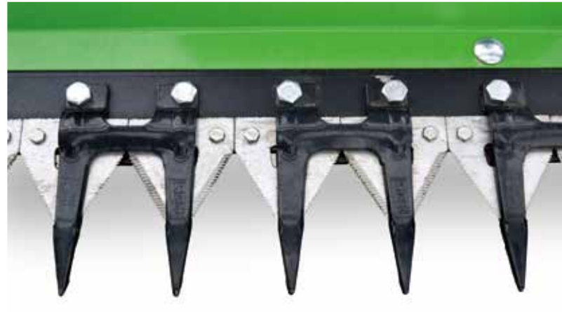
Knife sections mounted alternately cutting edge-up and cutting edge-down suffer less wear and ensure a clean cut every time.
