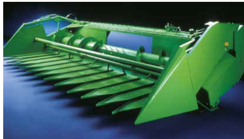
Sunflower attachment ensures that only seed heads are harvested, for maximum effectiveness of the threshing operation.
