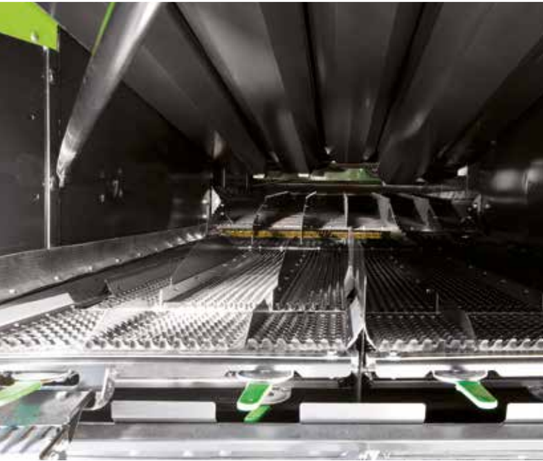
The cleaning system is top class in terms of sieving area and performance. With a cross flow fan and two-step cascade sieve, the 6040 is able to deliver levels of performance until now unknown in this segment of the combine market.
