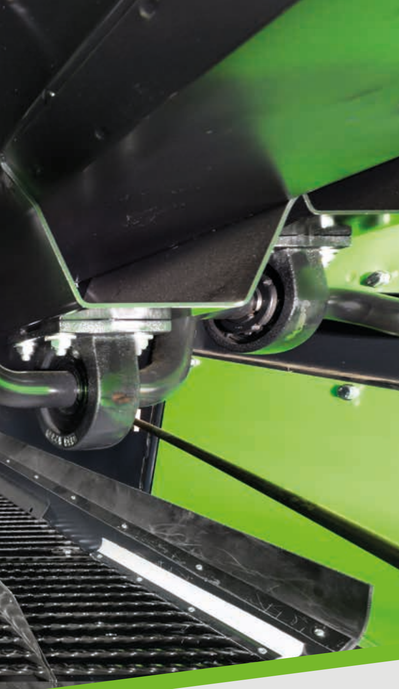
The cross-flow turbine ventilation system.
