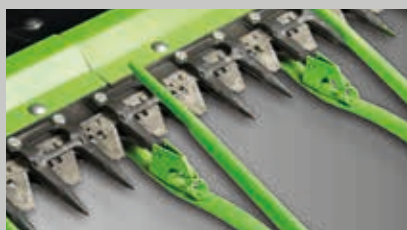
Patented Schumacher easy cut II knives.
