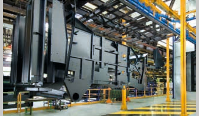
All components treated with cathaphoresis and automotive painting process.
