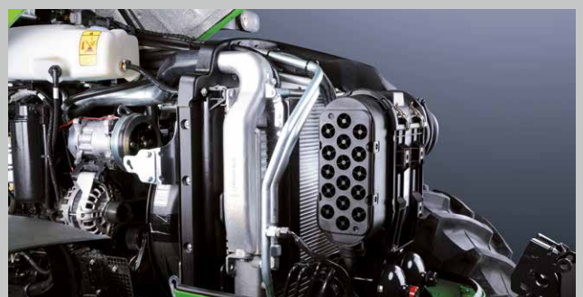
... the easy-to-clean cooling system with optional viscous fan.
