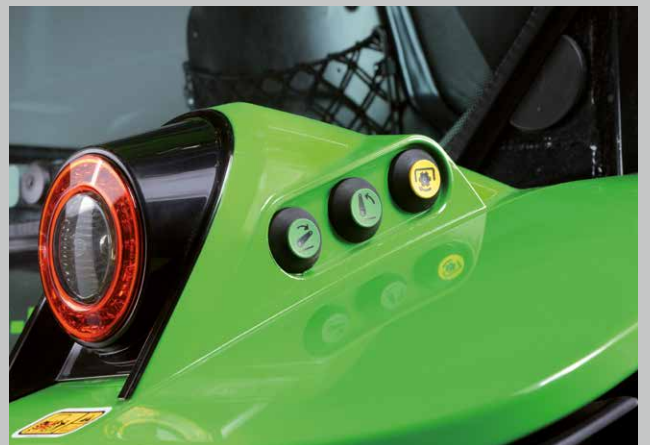
External PTO and linkage operation for easy device coupling and external PTO operation.
