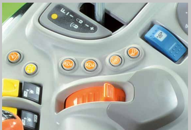
Two engine speeds can be saved. Efficiency preprogrammed for routine work.
