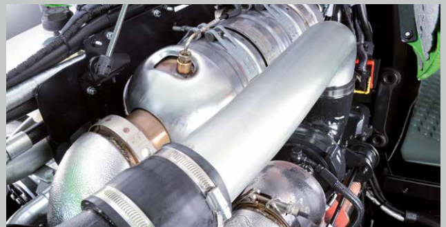
... DOC (Diesel Oxidation Catalyst) catalyst ensure lowest emission values.
