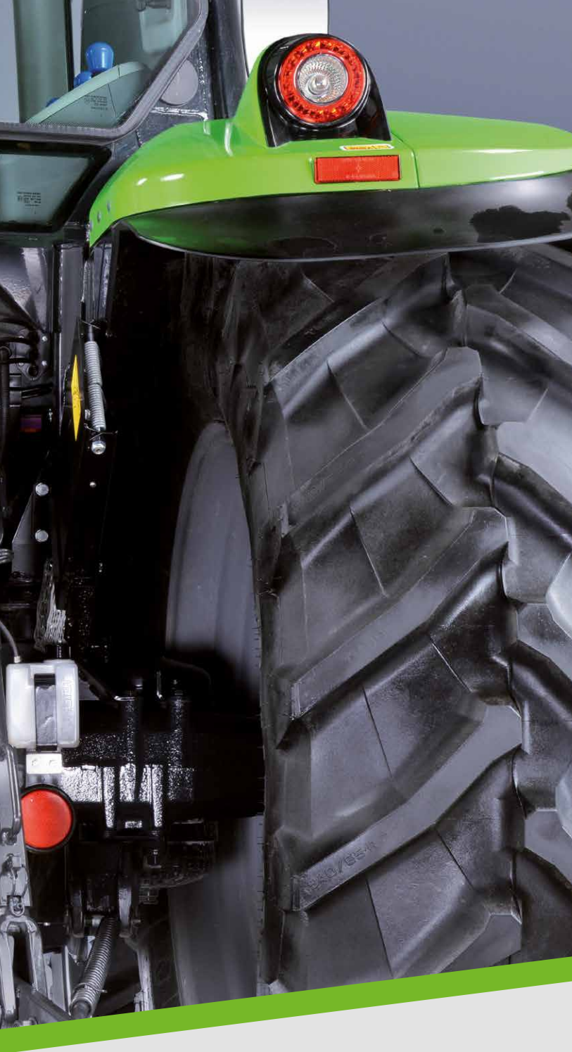
Front attachment area. 2,100 kg lifting power and 1,000 version PTO.
