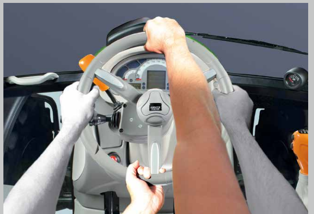
The SDD quick-steering system. Half steering wheel turn, double steering angle.
