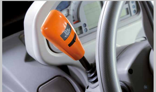
Powershuttle as a standard feature. Electrohydraulic powershuttle can only be set in 5 stages
