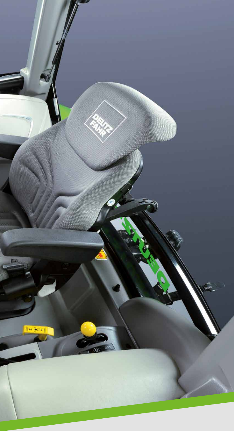
Up to 40% less vibration in the cab thanks to the Hydro-Silent block bearing.
