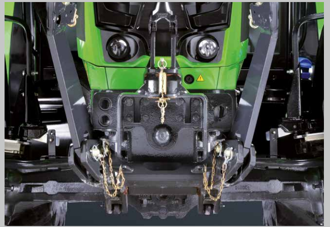
Front attachment area. 2,100 kg lifting power and 1,000 version PTO.
