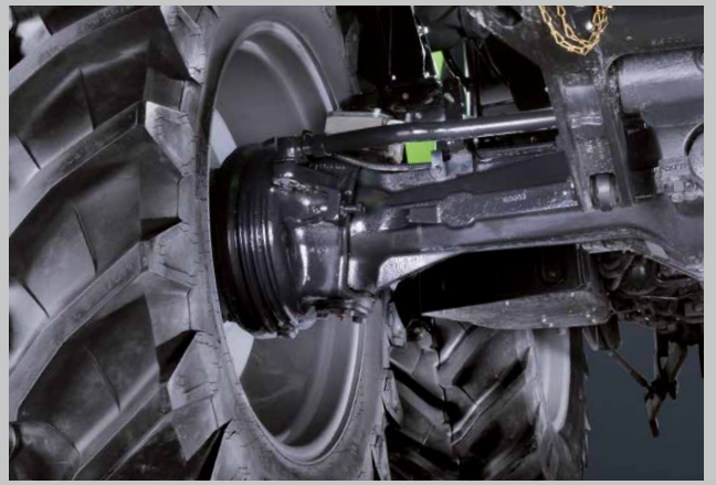
Unique safety concept of DEUTZ-FAHR. Separate oil-cooled disc brakes on the front wheels.
