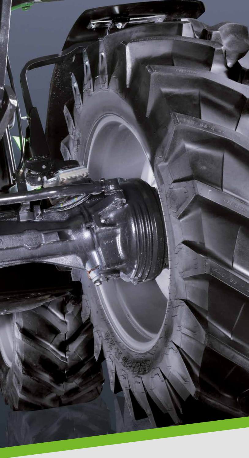
Unique safety concept of DEUTZ-FAHR. Separate oil-cooled disc brakes on the front wheels.
