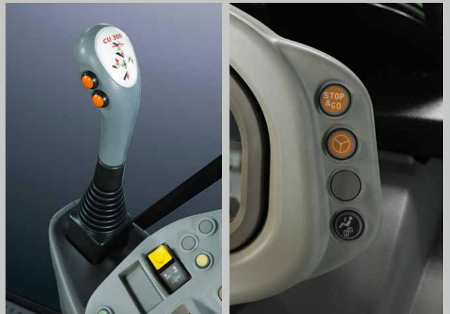
Front loader joystick with powershift buttons, Stop&Go and SDD quick steering system, and all...
