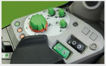
Precise draft and position control thanks to electronic rear lift on cab versions.
