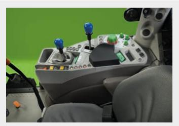
Rear spool valves controlled by single levers or mechanical cross lever.
