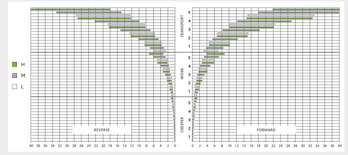
▲ HML transmission with 3-Powershift steps allows 45 speeds both in forward and in reverse direction.
