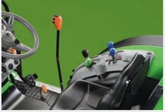
• Ergonomic side console with colour coded controls.
