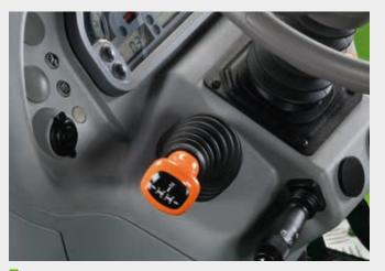
Ergonomic shuttle lever under steering wheel.
