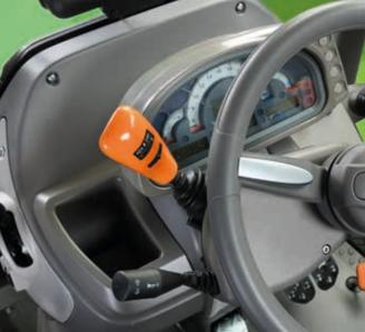
▲ PowerShuttle with SenseClutch 5-levels adjustment.
