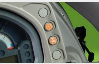
SDD function halves the number of steering wheel turning required for lock-to-lock steering.
