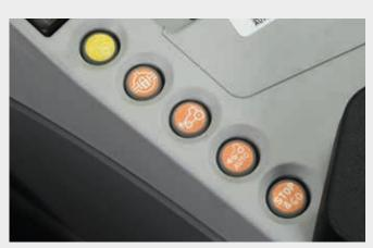
Auto 4WD function allows to engage and disengage automatically 4WD according to steering angle and speed.
