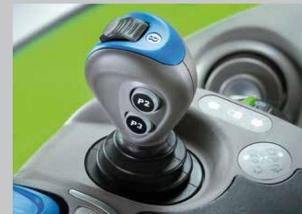
Hydraulic valves can be managed through proportional and programmable controls in terms of time and quantity. The electronic joystick can be programmed to use the front loader, whereas other tractor functions can be operated using the thumbwheel.
