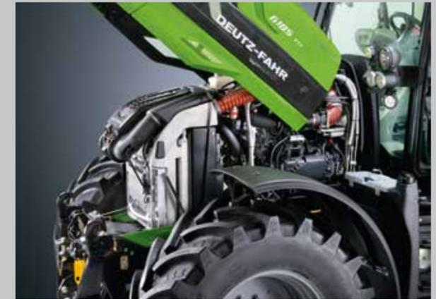
Highly efficient and compact cooling system with intercooler, engine, transmission, fuel cooler, and air conditioning condenser.
