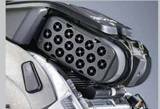
Precleaning system of the air intake filter: spiral cyclone tubes and an aspirator hose removes 95% of the dust before entering the primary filter.
