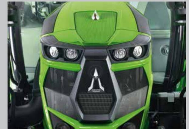
The 6 Series is standard equipped with halogen lights.
