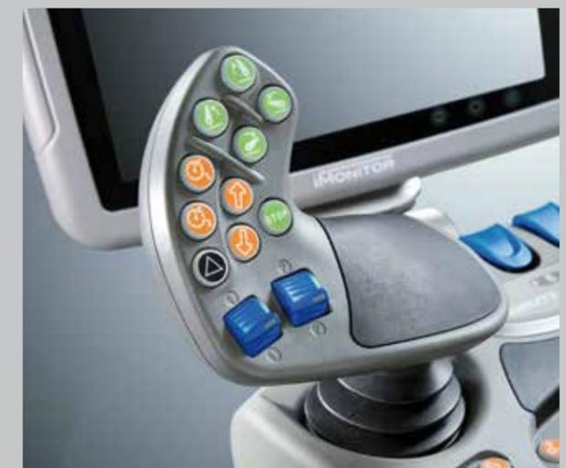
By simply pressing two buttons on the MaxCom multifunctional lever, the driver can recall four different speed settings whether in the field or on the road and maintain a constant speed for optimum results.
