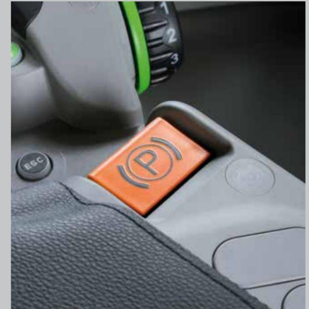
TTV models – EPB replaces the mechanical handbrake lever and is operated via an electric push-button control on the armrest console.
