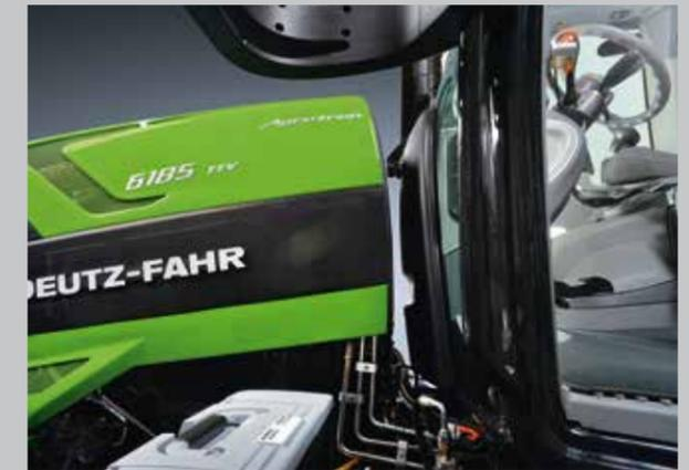
The cab and engine bonnet are separated from each other to significantly reduce noise and vibrations and thereby ensure maximum comfort.
