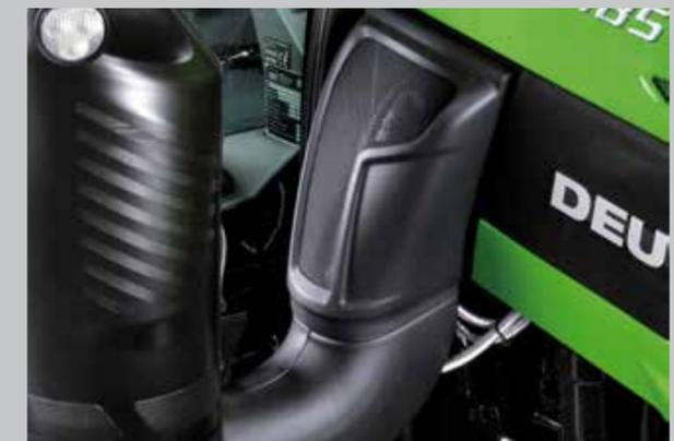
SCR after-treatment system and passive DPF (diesel particulate filter) is confirmed to be best solution in terms of performance, fluid consumption and maintenance.
