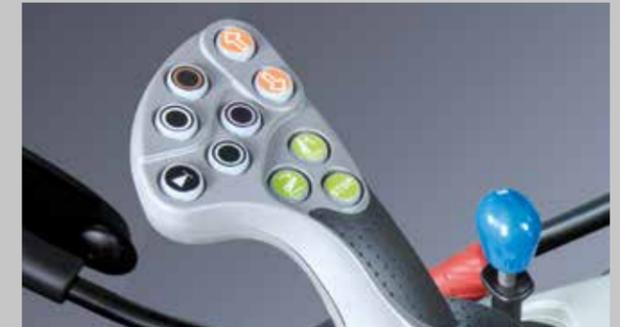
The TTV models are operated using the new PowerCom S joystick. Four buttons can be assigned to any function.
