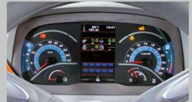
Cutting-edge instrument panel with new InfoCentre<sup>Pro</sup>: 5" LCD colour display and high resolution for a top-quality information concept customised by the user.
