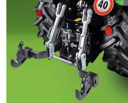
⬆ Electronically controlled rear linkage with a maximum lifting capacity of 2,600 kg.
