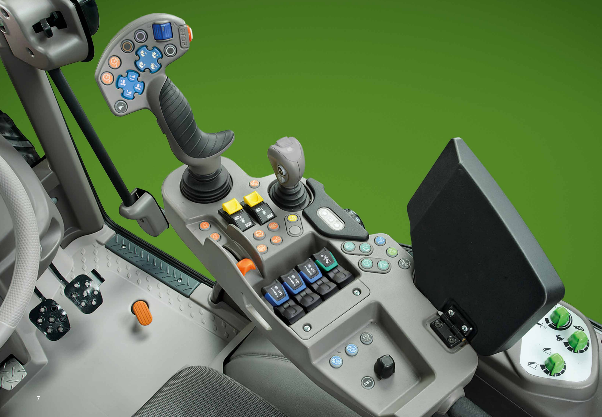
Clearly colour-coded fingertip and rotary buttons for intuitive handling and operation.
