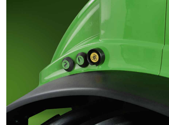
⬆ The rear linkage and PTO are operated with buttons in the rear wings.
