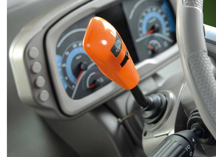
The direction of driving can be reversed with the individually adjustable powershuttle lever to the left of the steering wheel.
