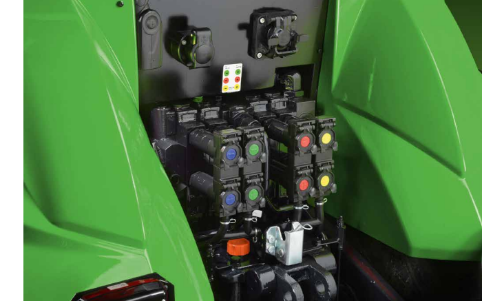
⬆ Five electro-hydraulically operated double-action control valves for easy tractor-based operation of attachments.
