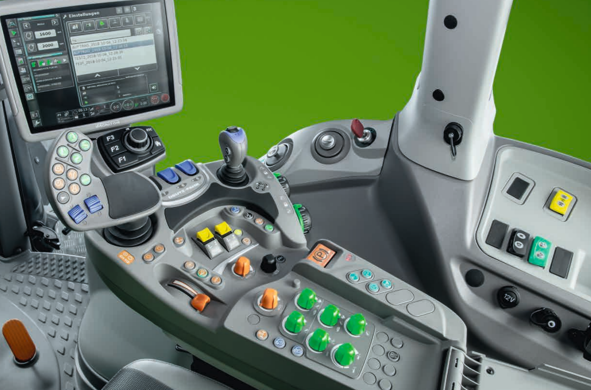
The PTO activation and engagement (front/rear) is integrated into the armrest ...
