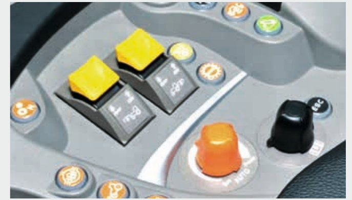
The PTO activation and engagement (front/rear) is integrated into the armrest ...
