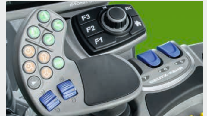
Four driving speeds can be stored and recalled for optimising work processes.
