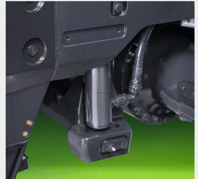
Unique new suspension concept for the front axle.
