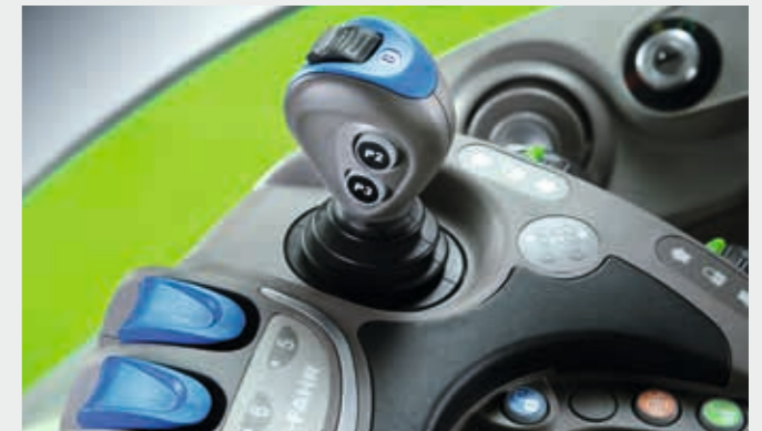
The hydraulic valves are actuated with a joystick with an integrated thumbwheel.
