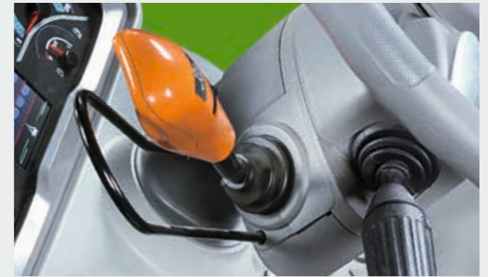
PowerShuttle and SensClutch can be used to easily adjust the response characteristics of the transmission.
