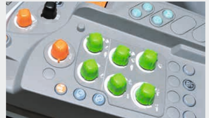
... as well as the controls for the front and rear linkage.
