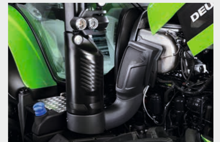
SCR exhaust gas treatment and passive DPF save fuel and operating costs.
