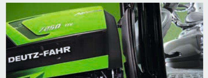
↑ Cab and bonnet are separated to reduce noise and vibration and increase comfort.
