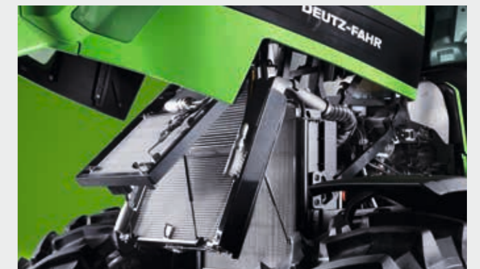
➤ The engine radiator can be opened and cleaned easily.
