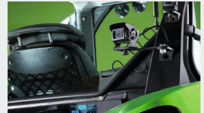
↑ Integrated camera with automatic full screen mode (e.g. reversing) for overview and safety.
