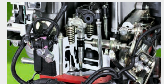
↑ DCR technology: 2,000 bar injection pressure ensures maximum engine efficiency.
