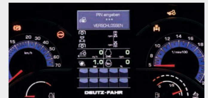
The new InfoCenter keeps the driver up to date: analogue and digital information about the operating status. Safety thanks to the code lock for the tractor. Lock and unlock with a PIN.
