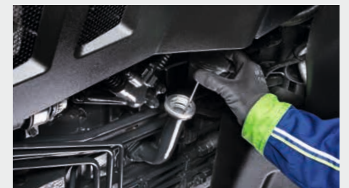
➤ Checking and topping up oil is very easy to do.
