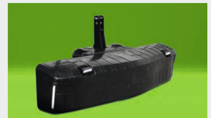
↑ Cast iron front ballast with up to 2,500 kg.
