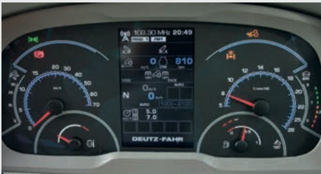
↑ State-of-the-art dashboard with InfoCentre PRO ; 5" high-resolution display. The available iLock system ensures security – lock and unlock the tractor with a PIN.
