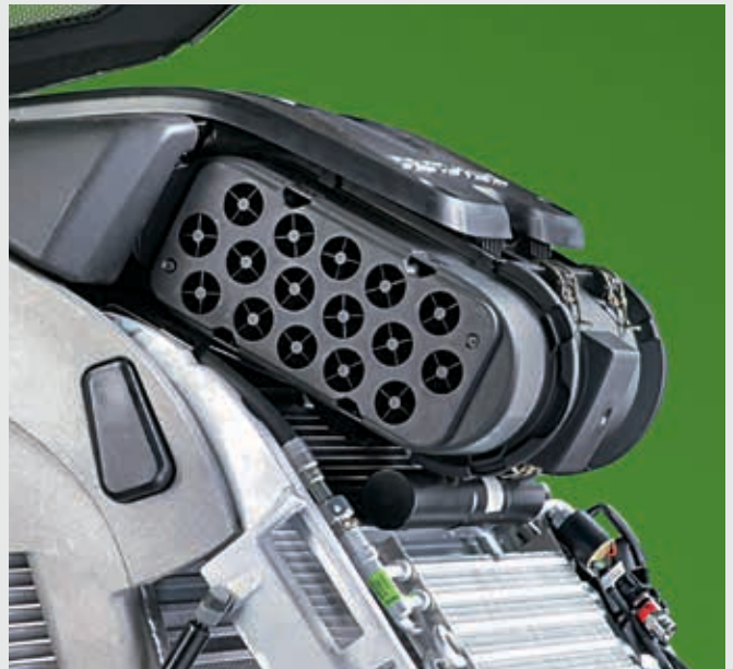
↑ Pre-cleaning system in the engine air filter: Spiral cyclone tubes and an aspirator hose remove 95 % of the dust before it can enter the primary filter.
