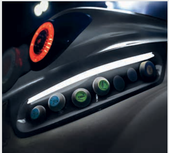
↑ LED illumination of mudguard controls.
