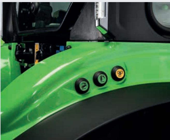
↑ External PTO and rear lift buttons on left and right fenders.
