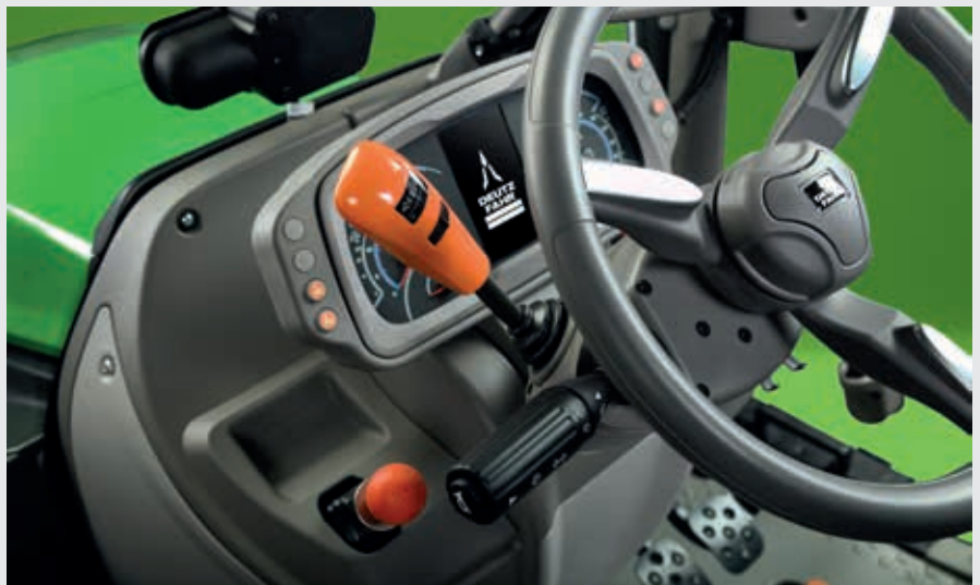
↑ PowerShuttle with SenseClutch (5 adjustable levels).
