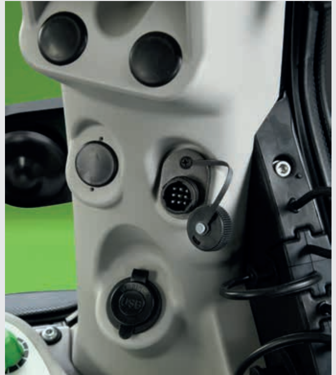
↑ In-cab ISOBUS plug for additional monitors.
