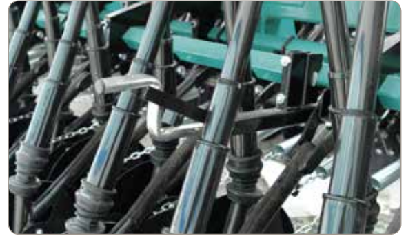
Centralized coulters adjustment.
