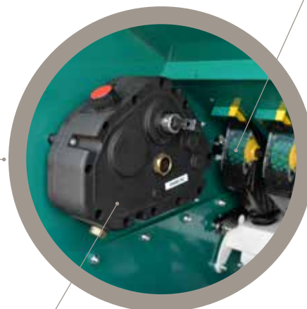
Additional variator for fertilizer or seed mixes
