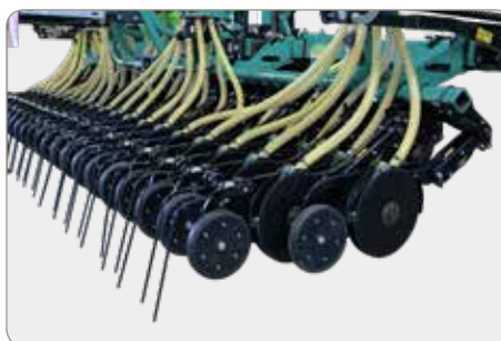
Seed-covering spring on wheel. Only for model with wheel.
