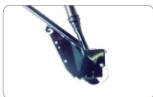
Suffolk coulters with depth control.
