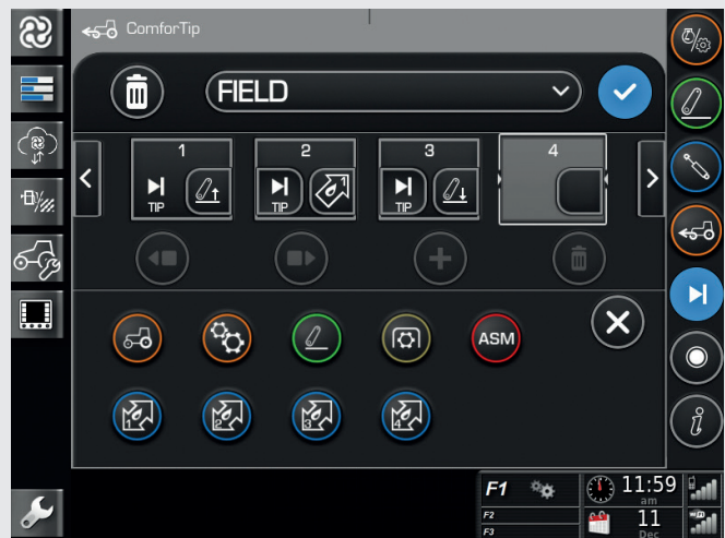
↑ Comfortip further increases the level of comfort. It allows recording of repetitive tasks and their recalling by pressing a single button.
