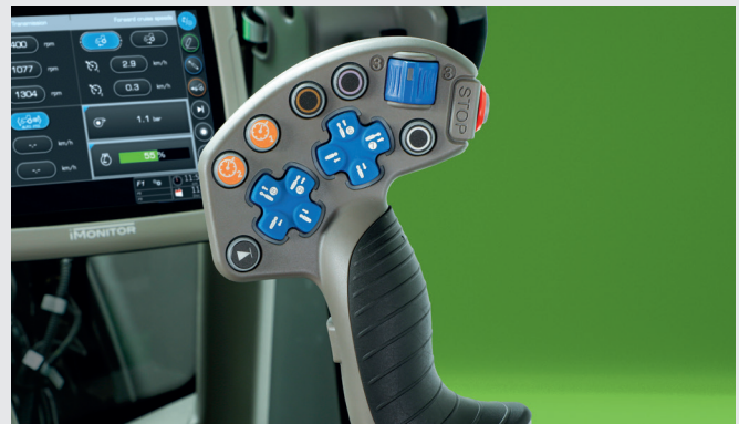
↑ MaxCom joystick for simple management of TTV transmission.
