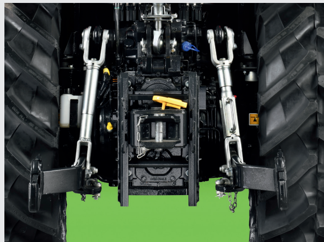
↑ Compact three-point hitch for narrow track.
