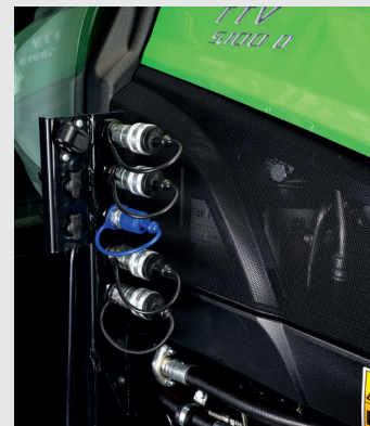
↑ Mid-mounted hydraulics ways for front implements.
