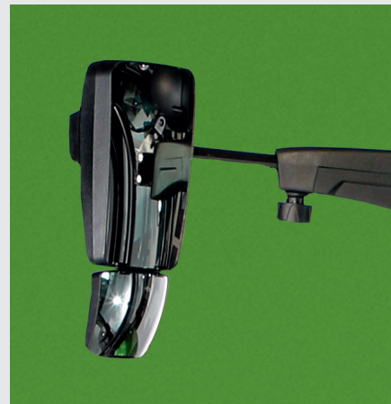
↑ Mirrors with electric adjustment and defrosting.
