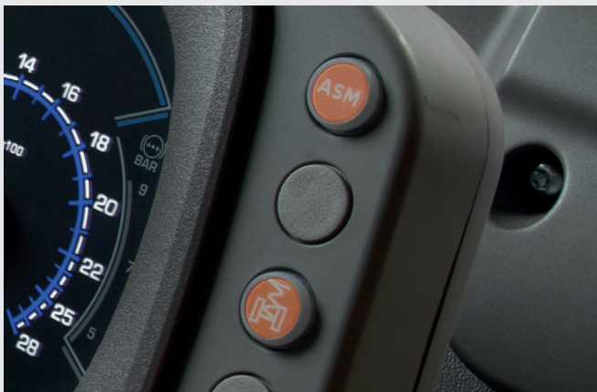
↑ ASM and front axle suspension activation.
