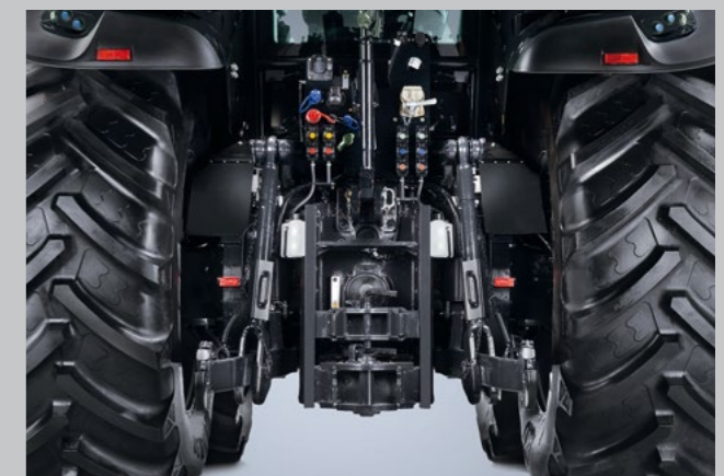
Hydraulic system output of up to 160 l/min, lifting capacity of 10,000 kg and four PTO speeds. Anything is possible.
