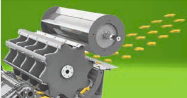
THRESHING DRUM, CONCAVE AND STRAW BEATER. A broad 600 mm diameter threshing drum measuring 1.27 m in width for the 5 straw walker model and 1.52 m in width for the 6 straw walker model, and a multi-segment concave with a pitch of 121° ensure perfect threshing results in all conditions.
