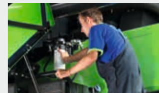
Fuel tank and filters. Easy to clean fuel tank area and replace filters.
