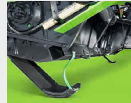
The sensor skids allow the header to follow the contours of the terrain precisely and make instant adjustments to ensure an even cutting height.
