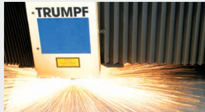
Every part of the combine structure is produced with the use of Laser cutting machines which, starting from the 3D drawing, allow the finished piece to be made.
