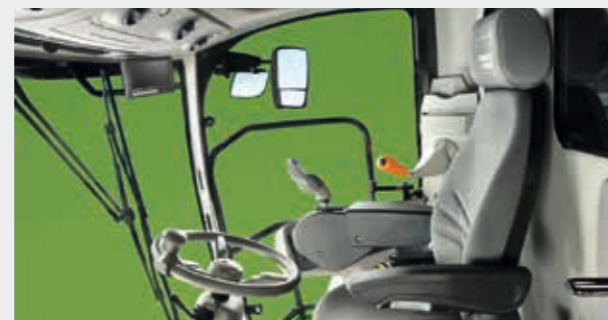
Ergonomic seat with mechanical or pneumatic adjustment and adjustable steering column for setting a comfortable driving position.
