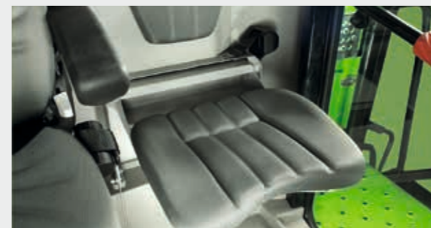
PASSENGER SEAT. Folds for optimal usage of space in the cab.
