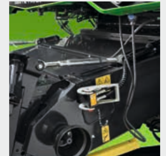
↑ Adjustable cutting angle for following the contours of uneven terrain perfectly.
