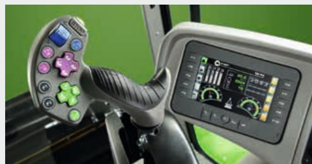
COMMANDER STICK. For controlling: 1) Position and inclination of header
