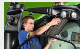
Cab filters. Easy to replace cab air filters with no tools required.
