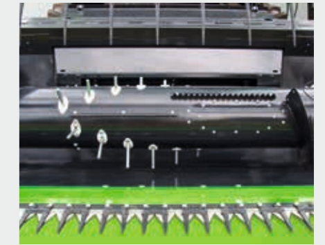
The feeder auger with full length retractable fingers ensure continuous feed and crop flow.
