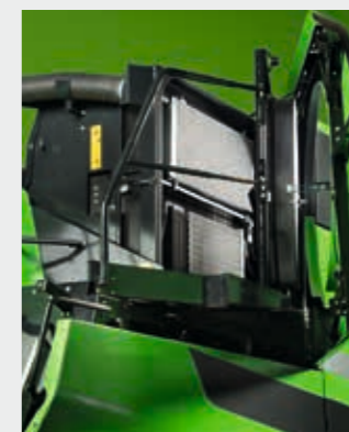
Access for radiator cleaning.
