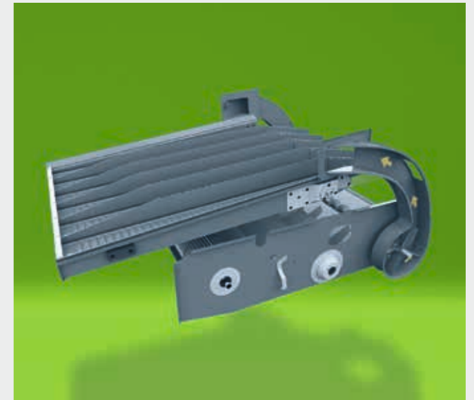
⚙️ An overload safety system ensures excellent reliability. The dual grain return system (DGR) has two different operating speeds selectable in relation to the crop processed to ensure complete grain care in all conditions.
