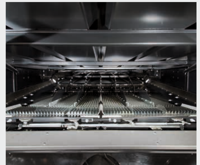
⚙️ An (optional) electrically operated sieve adjustment system lets the operator adjust sieve clearance instantaneously in relation to harvesting conditions.
