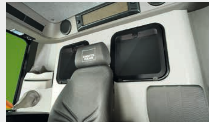
↑ Visual grain tank monitoring. A double window in the cab lets the operator visually check the fill level of the tank and the quality of the grain harvested.
