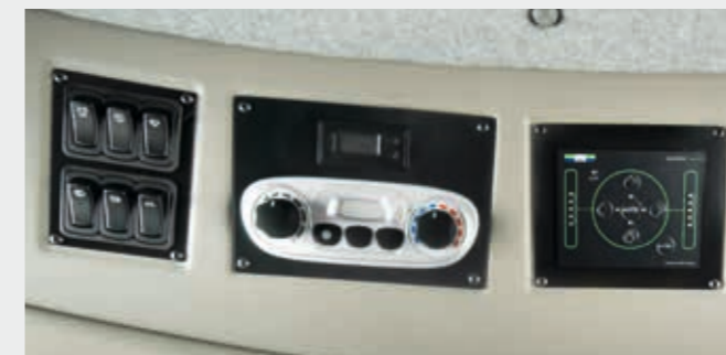
↑ The Balance system adjusts the position of the entire machine completely automatically to correct for lateral gradients up to 20% and longitudinal gradients up to 6% and keep the combine harvester perfectly level.
