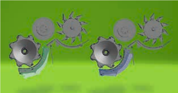
CONCAVE ADJUSTMENT. The clearance between the concave and the threshing drum at the input and output can be independently adjusted at the front and rear via electric actuators controlled by the Commander Control.
