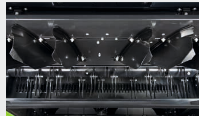
↑ Straw Chopper, for even more effective material distribution, the straw chopper may also be equipped with deflectors, adjusted electrically from the cab, to adjust spreading to weather conditions.
