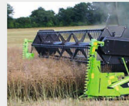
The rapeseed kit may be fitted to the grain header for even greater versatility.
